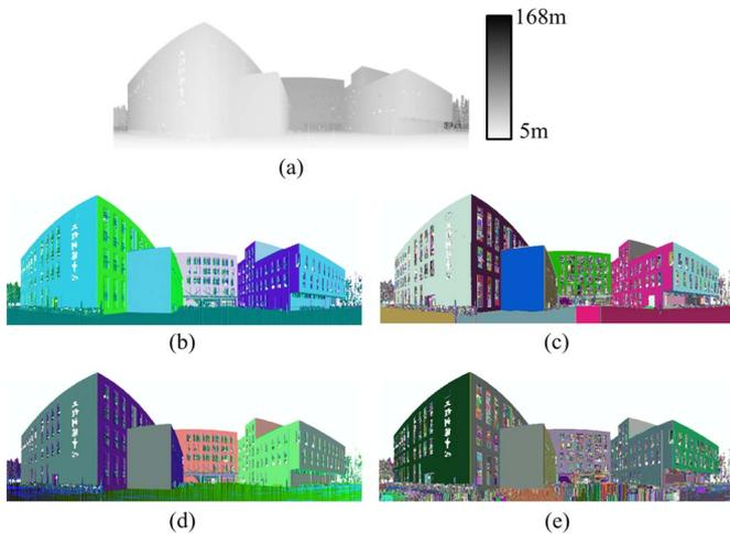
Fig. 2. Planar segmentation of a building. (a) Range image. (b) Synthetic image of planar parameters  $(\rho, n_x, n_y)$ . (c) Segmented image using the synthetic image in (b). (d) Synthetic image of planar parameters  $(\rho, \theta, \phi)$  using the method in [8]. (e) Segmented image using the synthetic image in (d).
