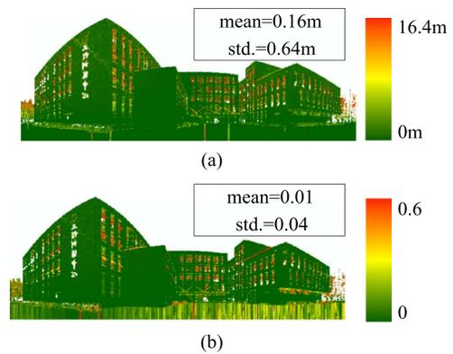
Fig. 3. Difference images of planar parameters computed using our proposed method and the method in [8]. (a) Difference image of planar parameter  $\rho$ . (b) Difference image of the normal vectors. The lengths of the difference normal vectors are shown.
