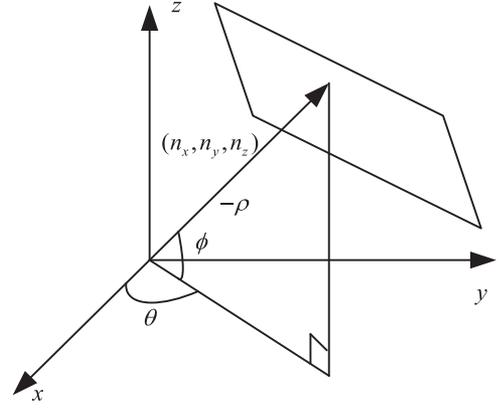
Fig. 1. Planar parameterization using the three components of the normal vector versus using the horizontal and vertical angles of the normal vector.
