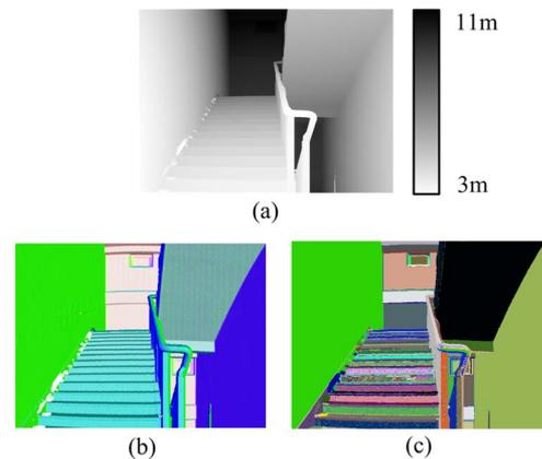
Fig. 4. Planar segmentation of a staircase. (a) Range image. (b) Synthetic image of planar parameters  $(\rho, n_x, n_y)$ . (c) Segmented image using the synthetic image in (b).
