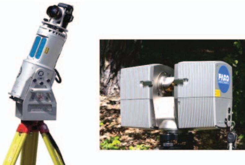
Figure 2. Riegl LMS Z420i and FARO LS 800 HE80 terrestrial laser scanner instruments.
