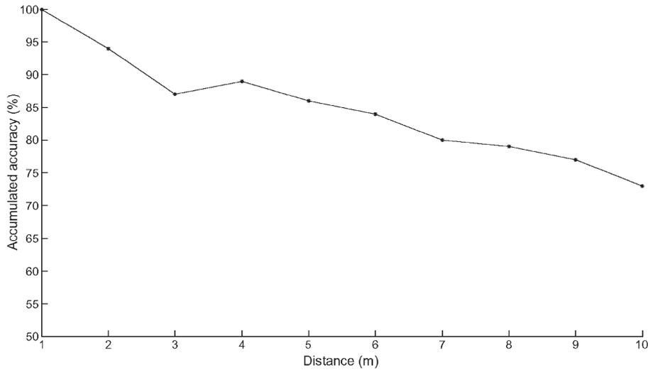
Fig. 5. Stem-locating accuracy as a function of range.
