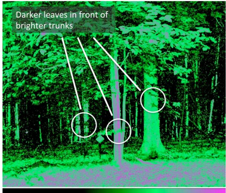
Figure 2. DWEL scan at Harvard Forest, SWIR laser. Color bar indicates returned power, low to high, left to right.
