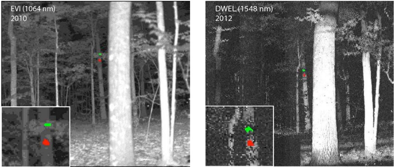
Figure 3. Left, EVI scan at 1064 nm. Right, DWEL scan at 1548 nm. Image brightness is proportional to returned power.
