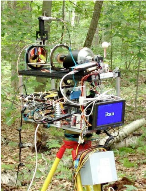
Figure 1. DWEL instrument in engineering scan configuration.
